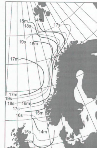
Figure 6.2.1 Significant wave height H_{m0} and related maximum peak period T_P with annual probability of exceedance of 10^{-2} for sea-states of 3 hours duration. Isocurves for wave heights are indicated with solid lines while wave period lines are dotted.
